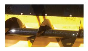
4. Remove the three bottom bolts from the access cover. Install AGTNHD2170 using the three bolts for the bottom of the access cover as shown Slide the liner to the left So that the left end is against the vertical lift auger housing. Note: the poly liner should not overlap the access cover; it should just come up to the edge of it.
