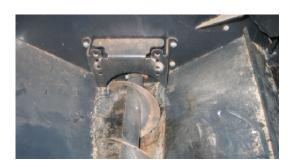
2. Remove patches/repairs that would restrict the poly liners from laying flat against the top surface of the metal trough.
