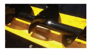
3. Start with Lower auger trough: Insert Liner (AGTNP10100) under the auger and use shims to wedge panel down tight against floor as shown in the picture to the right. Be sure the panel is inserted so the shape of the liner matches the trough.
